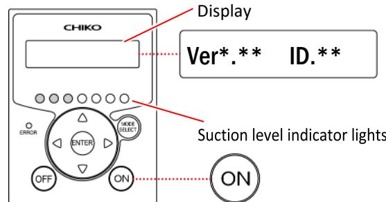
Note: The control panel will not respond during a remote connection.
