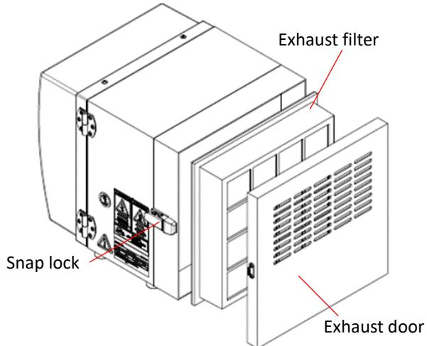
2. Remove the exhaust filter.
