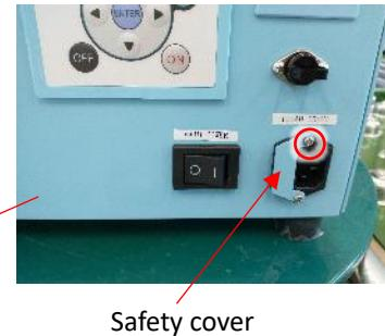
2. Replace the fuse according to "6.5".
