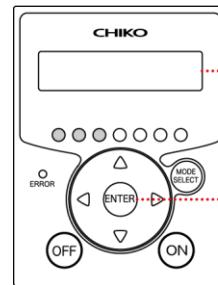
4. When the display shows “Reset Runtime Y”, press [ENTER].
