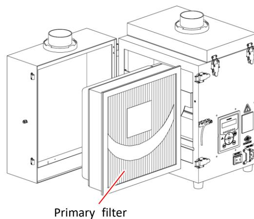
4. Make sure that an O-ring is seated on the new primary filter.
