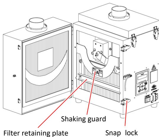
Shaking guard      Filter retaining plate      Snap lock
