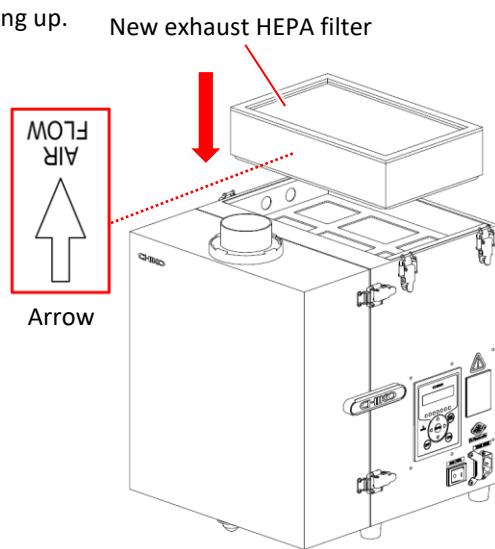
6. Install the exhaust port cover and secure them with the snap locks on both side.
