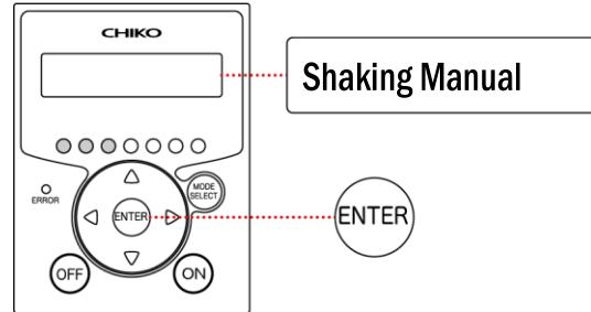
4. Check that [Shaking Start Y] is shown on the display, and press [ENTER]. This starts shaking operation.
