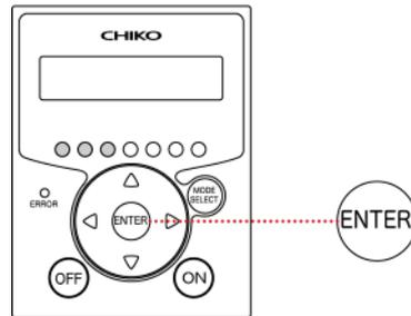
3. When the display shows “Initial DP Get Y”, press [ENTER]. The machine now begins acquiring initial pressure. Wait until the registration process is complete.
