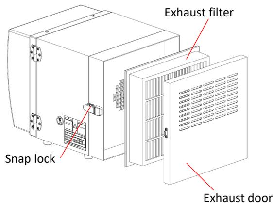
2. Remove the exhaust filter.
