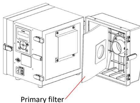
4. Install the new primary filter and install the secondary filter back in place.
