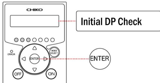
4. Once the initial pressure is registered, the display shows “Initial DP Entry”, and the machine returns to normal operation.
