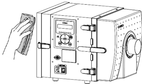
2. Release the snap locks and open the intake filter chamber.
