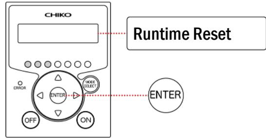
4. When the display shows “Reset Runtime Y”, press [ENTER].
