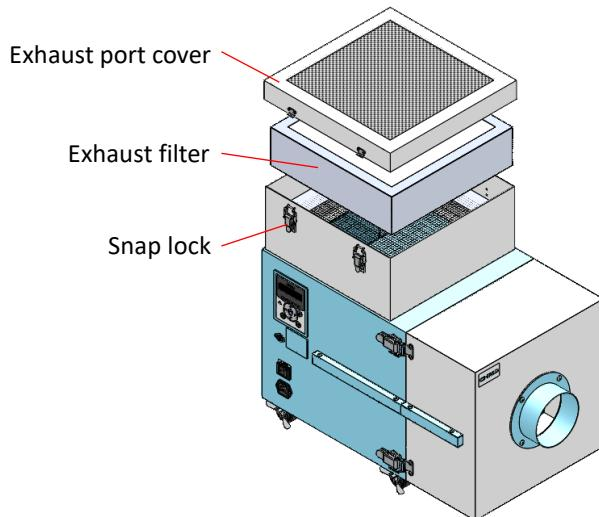
3. Install the new exhaust filter.
