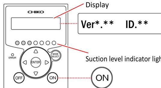
Note: The control panel will not respond during a remote connection.
