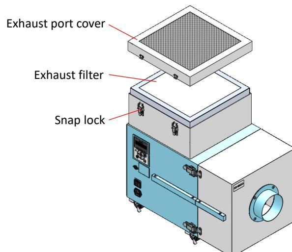
2. Remove the exhaust filter.
