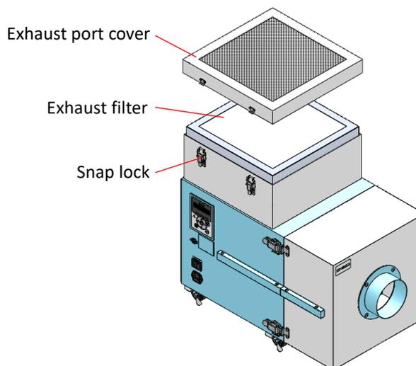
2. Remove the exhaust filter.
