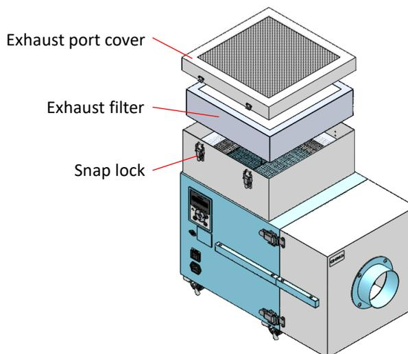
3. Install the new exhaust filter.
