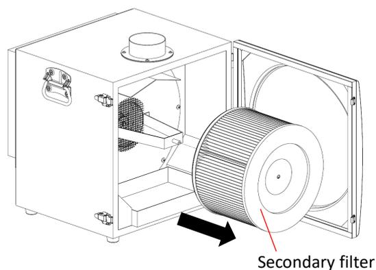
5. Install a new secondary filter and install the primary filter back in place.
