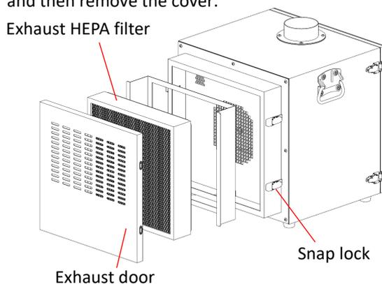
2. Remove the exhaust HEPA filter.
