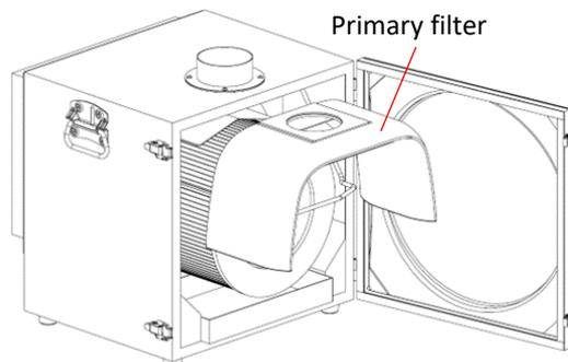
4. Insert the gasket of the new primary filter firmly into the cylinder pipe and restore it as before.
